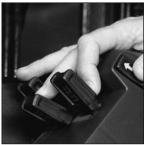
Fingertip hydraulic controls
